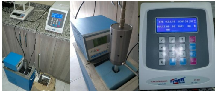
Figure 2. Preparation of nanofluid with temperature control
