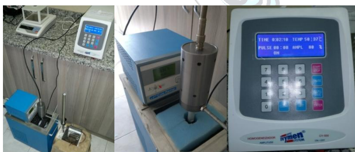
Figure 2. Preparation of nanofluid with temperature control
