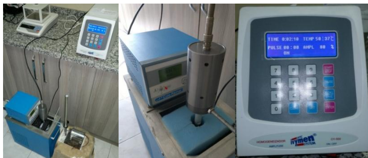
Figure 2. Preparation of nanofluid with temperature control
