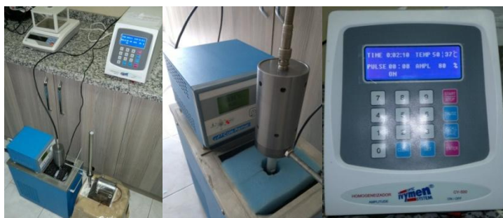
Figure 2. Preparation of nanofluid with temperature control
