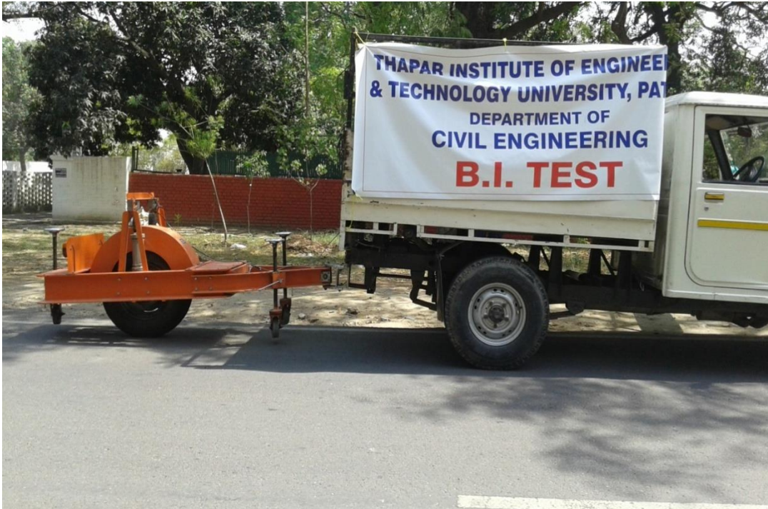
Fig. 1. Bump integrator test (Roughness test)
