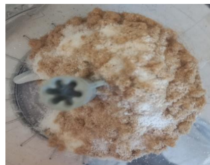
Figure 2. Jute and powder PLA mix, before entering the mixer.
