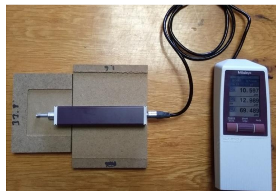
Figure 3. The measurement of the surface roughness with roughness tester
