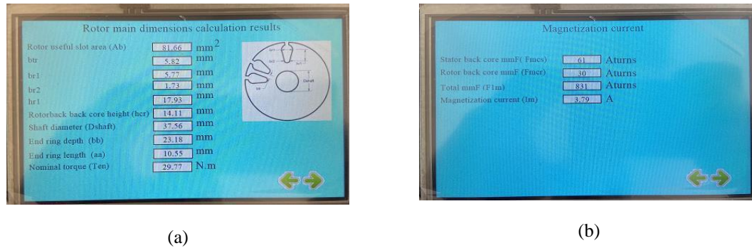
Figure 15. Application circuit screen view of rotor main dimensions calculation results (a) and magnetization current (b)
