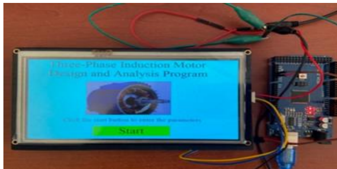
Figure 5. Application circuit consisting of Arduino mega and Nextion screen
