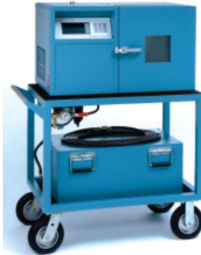
Figure 1. The two-pressure humidity generator
