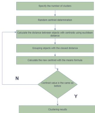
**Figure 2.** General process of the K-means algorithm
