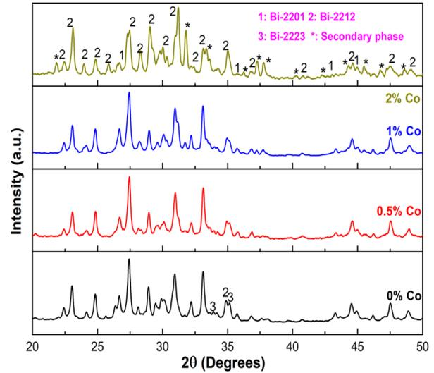
**Figure 1.** XRD patterns of  $\text{Co}_3\text{O}_4$  nanoparticles-added Bi-2212 ceramics
