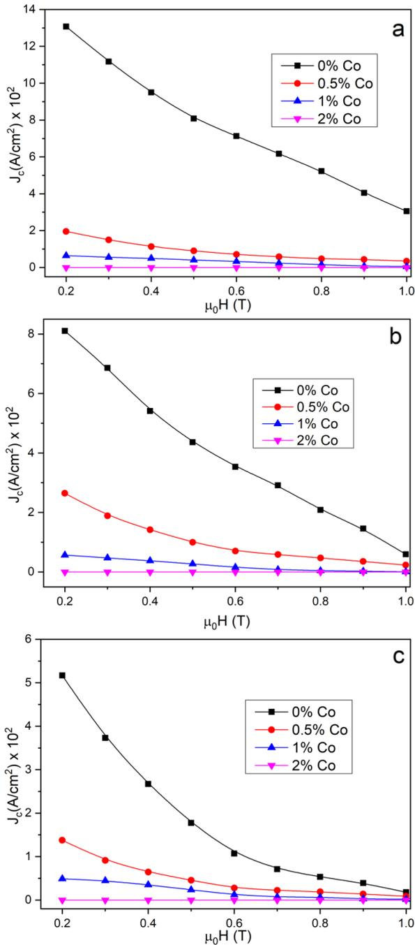
**Figure 5.** Critical current density versus magnetic field for a) 10 K, b) 15 K, and c) 20 K
