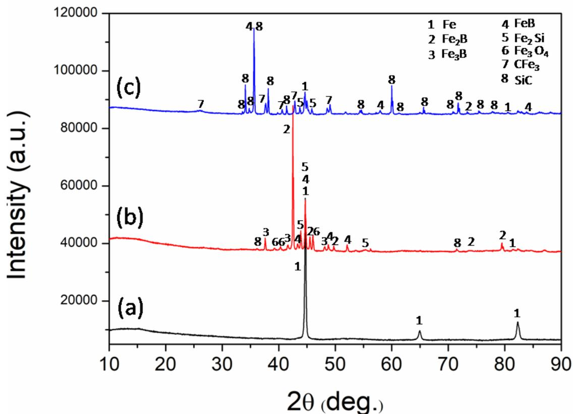
**Figure 2.** XRD pattern of (a) 1018 steel, (b) 2h boronized, (c) 4h boronized steel
