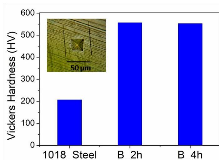
**Figure 6.** Vickers hardness of the samples. The inset picture shows the imprint image after indentation
