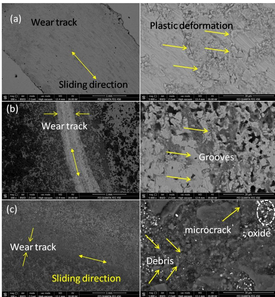
Figure 5. Worn surface of the samples (a) Untreated steel, (b) 2hboronized, (c) 4hboronized (100x and 5000x magnification)
