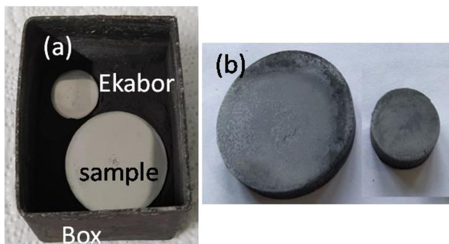
**Figure 1.** Samples (a) Before boronizing and (b) After boronizing
