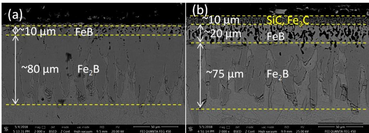
**Figure 3** BSE images of boronized steel (a) 2h and (b) 4h
