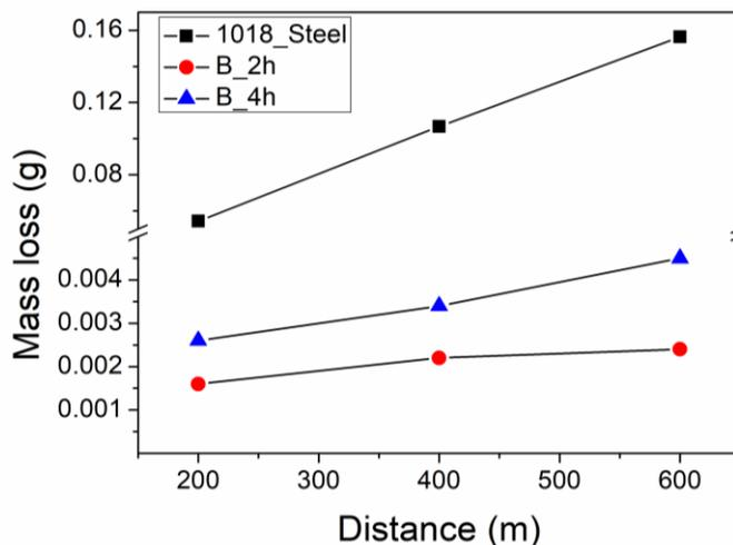
Figure 4. Mass losses of the samples for different sliding distances
