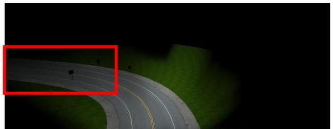
Fig.34. Simulation LB + V5 Cornering/Bending module
