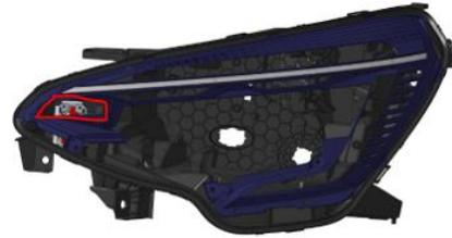
Fig.4 Location of FBL module in the headlamp
