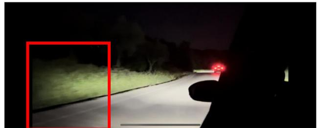
Fig.38. Night Drive test: low beam+ cornering/bending module
