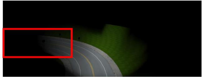
Fig.33. Simulation Low Beam distribution on the bending road
