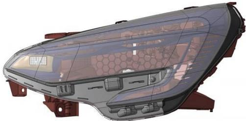
Fig.20. 3D of the Cornering/Bending Module in the Headlamp
