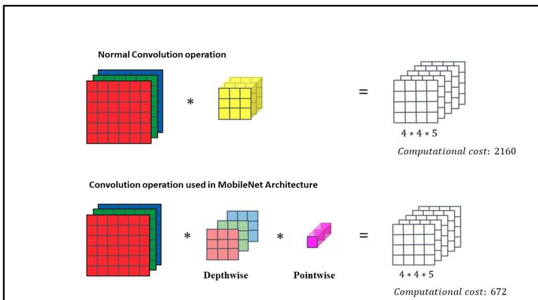
**Figure 5.** The difference between the convolution operation used in the MobileNet architecture and the normal convolution operation.
