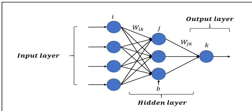
**Figure 2.** General representation of artificial neural network.
