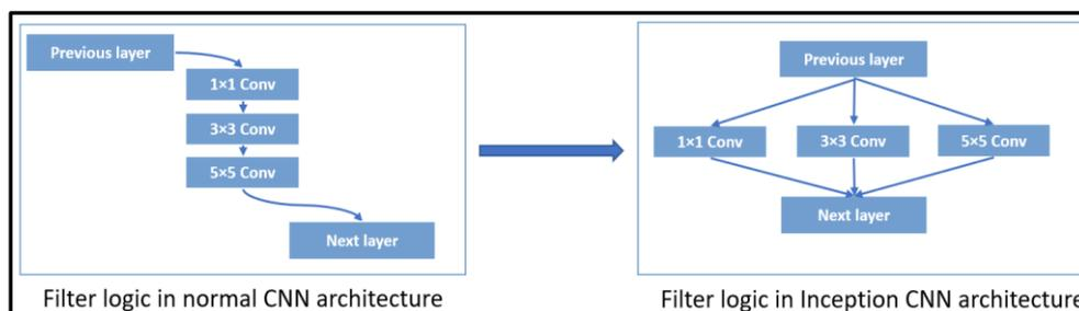
**Figure 4.** Filter logic used in the Inception architecture.
