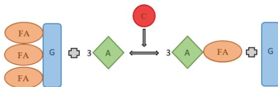
Fig. 2. Schematic illustration of transesterification reaction. (FA: Fatty Acid, G: Glycerin, A: Alcohol, C: Catalyst [22].
