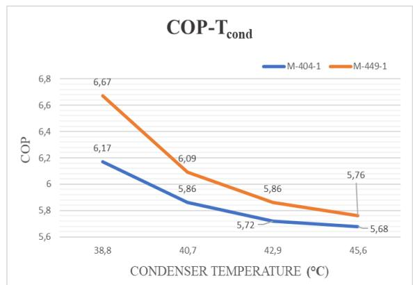
Figure 8. Condenser temperature and COP variation for single-stage refrigeration
