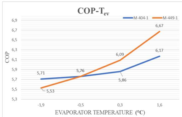
**Figure 9.** Evaporator temperature and COP variation for single-stage refrigeration
