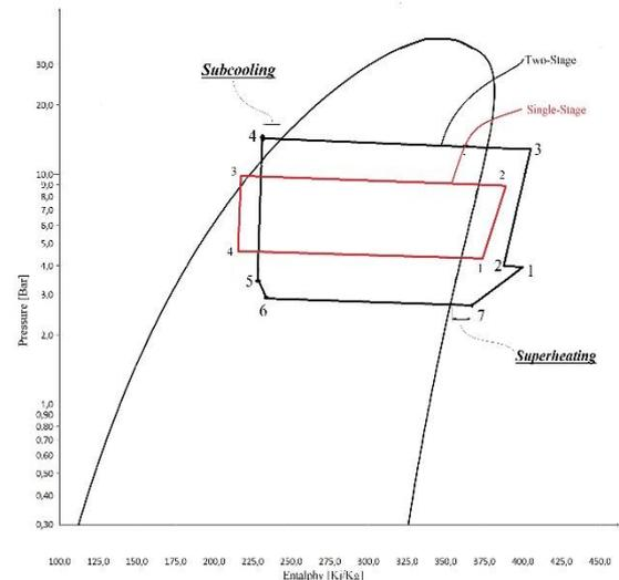
**Figure 2.** Pressure-enthalpy diagram of the cycle
