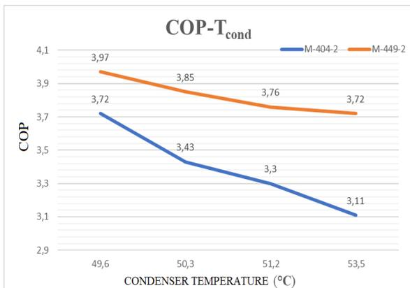
Figure 6. Condenser temperature and COP variation for two-stage refrigeration
