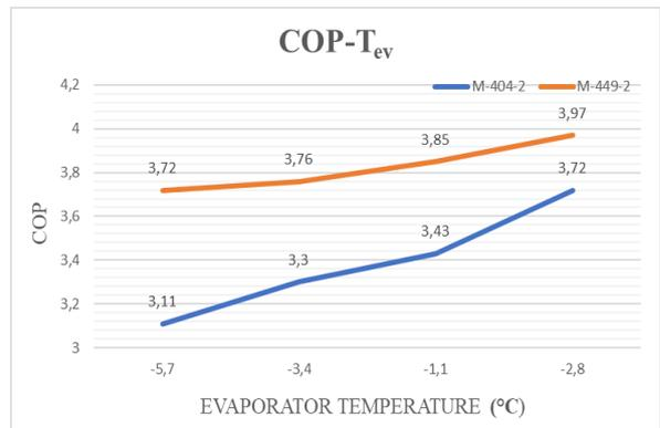
Figure 7. Evaporator temperature and COP variation for two-stage refrigeration
