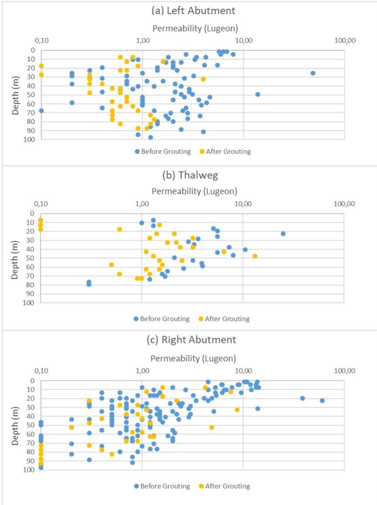
**Figure 11.** Comparing permeability before and after grouting at the dam axis [23].
