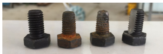
Figure 4. Accelerated and artificial corrosion of the bolts
