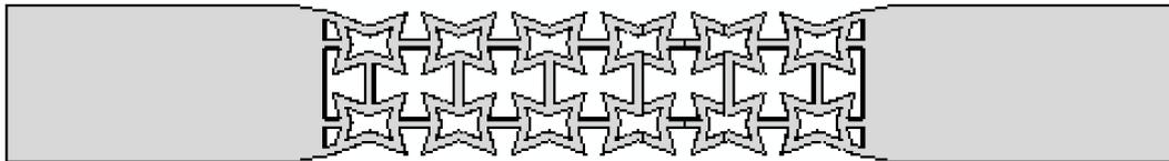
**Figure 4.** Geometry of auxetic structure to investigate the tensile behavior of samples made by DMLS method
