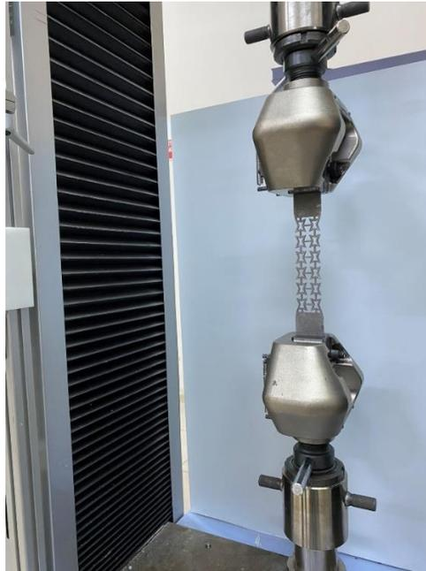
**Figure 3.** Tensile test setup
