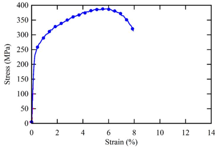
Figure 5. Stress-strain curves of AlSi10Mg alloy obtained from the tensile test
