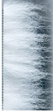
Figure 3. Bundle of fibres extended from HVI clamp.
