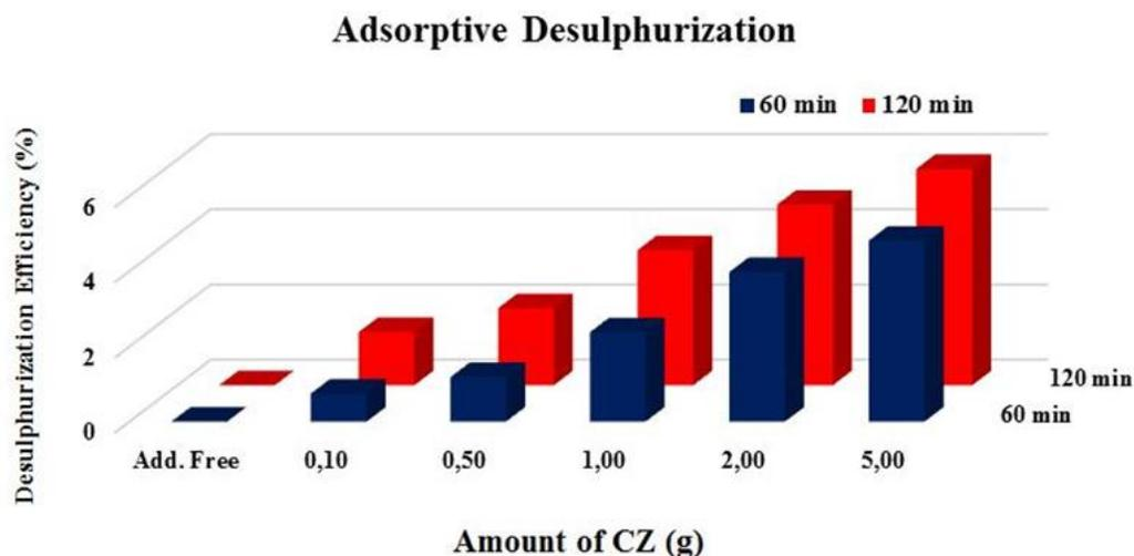
Figure 2. The impact of CZ contact time and quantity on adsorptive desulphurization
