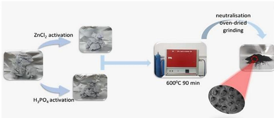
Figure 1. Production of activated carbon from waste paper
