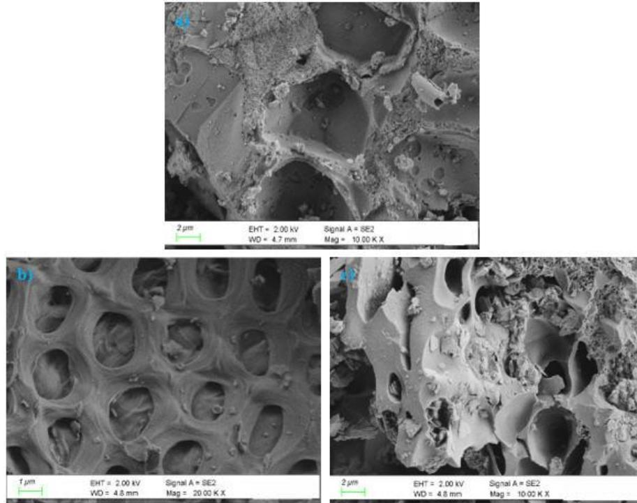
Figure 3. FE-SEM images of (a) Commercial activated carbon, (b) WPA and (c) WPS activated carbons
