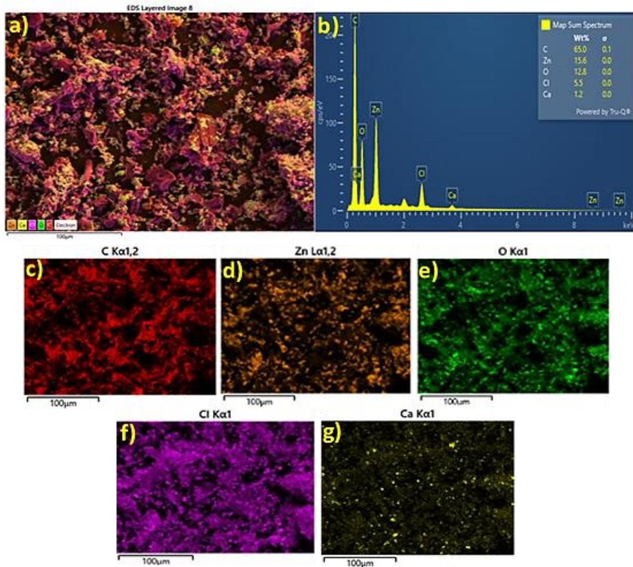
Figure 6. FE-SEM Mapping and EDS analyses of activated carbon produced from waste paper by using zinc chloride ( $ZnCl_2$ ) as activation agent
