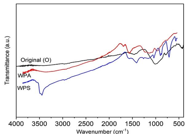
Figure 2. FT-IR spectrum of activated carbons
