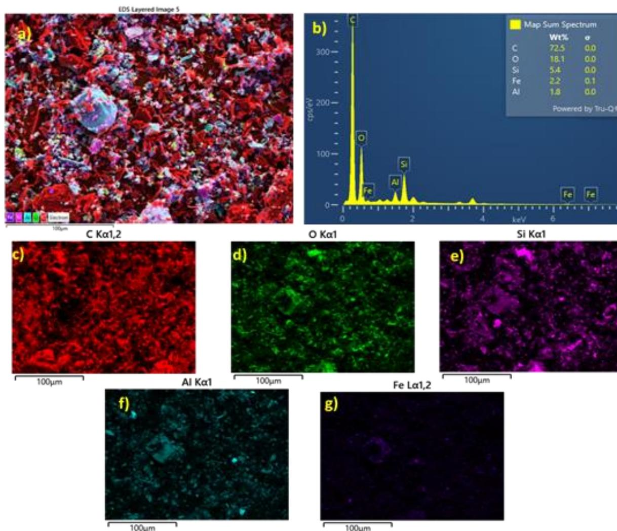
Figure 5. FE-SEM Mapping and EDS analyses of the activated carbon produced from waste paper by using phosphoric acid ( $H_3PO_4$ ) activation agent
