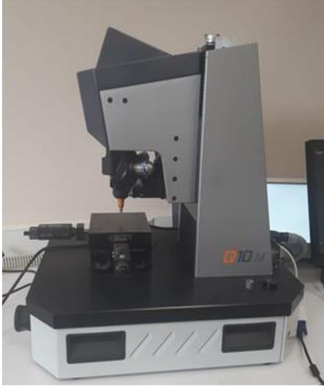
Figure 3. Microhardness tester.
