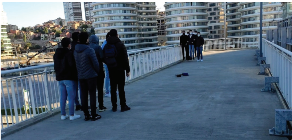
Figure 13 - Application of jumping protocol with five students on points J1 and J2
