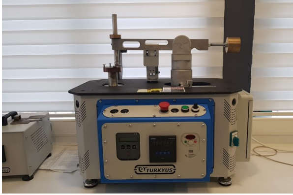
Fig. 1. Pin on disc wear tester.
