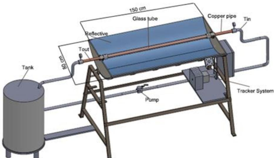
**Figure 2.** Parts of the parabolic collector
