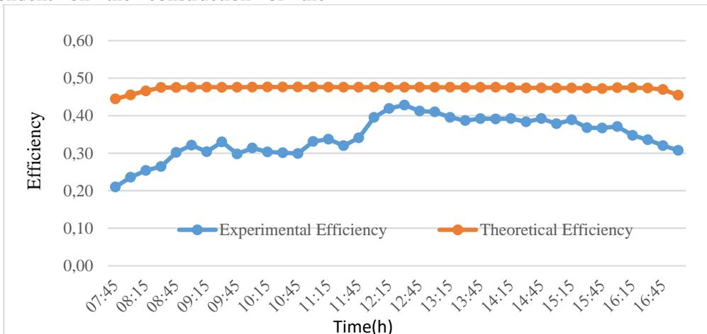
Figure 4. Theoretical and experimental thermal efficiency
