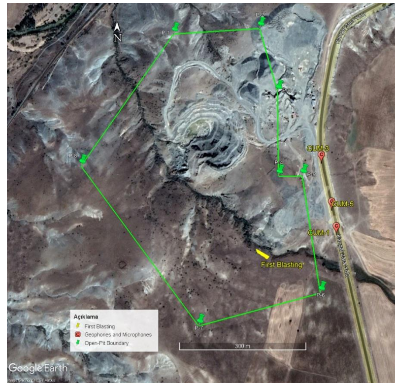
Figure 6. Measurement points of ground vibration and air blast (First blasting).
