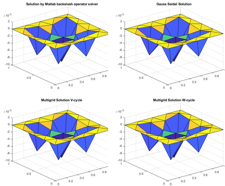
FIGURE 2. Solution of (25) on fine grid using M.B.O, G.S, M.G V-cycle and W-cycle after 100 iterations.
