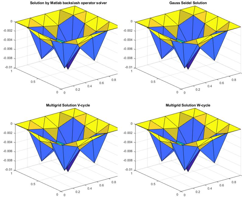
FIGURE 4. Solution of (26) on fine grid using M.B.O, G.S, M.G V-cycle and W-cycle after 100 iterations.
