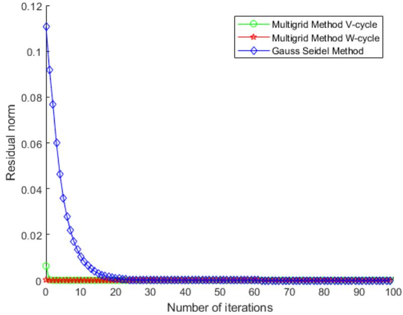
FIGURE 1. Comparison between the convergence of maximum residual norm by M.G and G.S.
