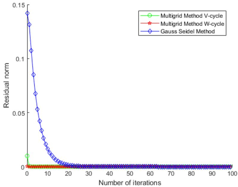
FIGURE 3. Comparison between the convergence of maximum residual norm by M.G and G.S.
