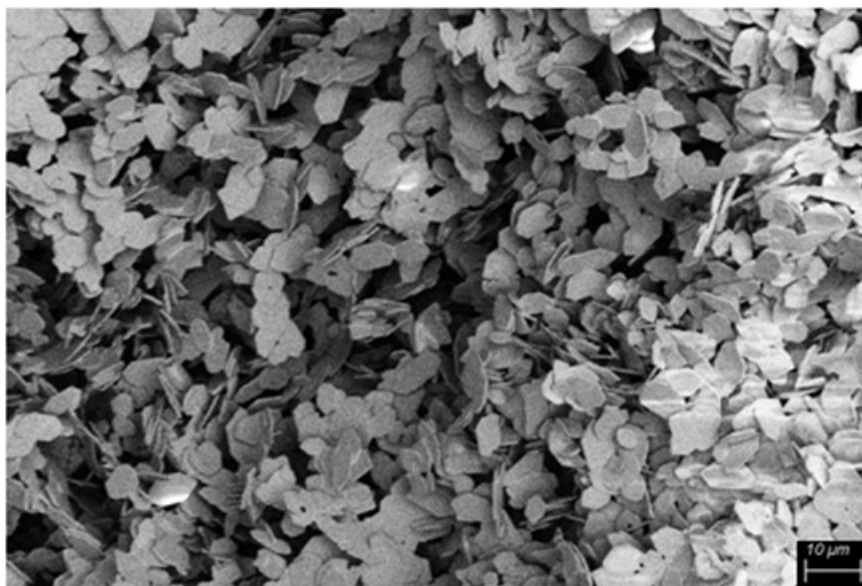
Figure 4. SEM image of copper hydroxynitrate.
