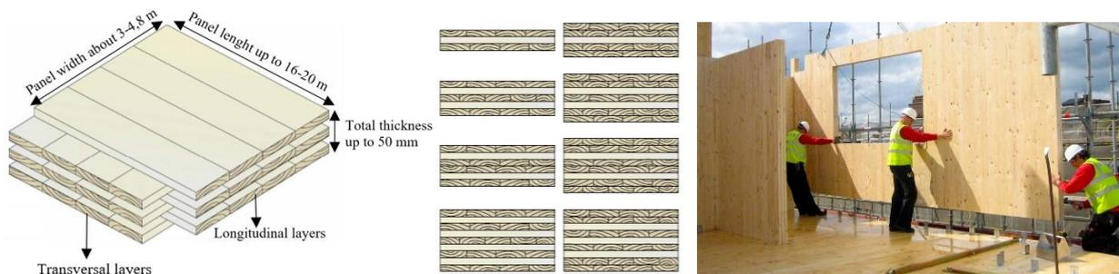
**Figure 1.** CLT panel section [13] and application in buildings [14]
