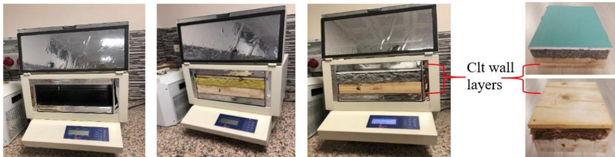
**Figure 3.** Measurement Examples Made on The LaserComp Fox-314 Thermal Conductivity Device
