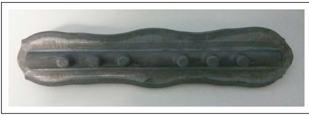
Figure 14. Sample with flash (Case-14, 1150 °C-3.5 mm-38 RSB).
