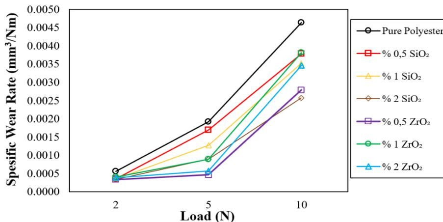
**Figure 4.** Variations of the wear rate of nanoparticle reinforced polyester composites at 1 m/s depending on the reinforcement ratio and the load
