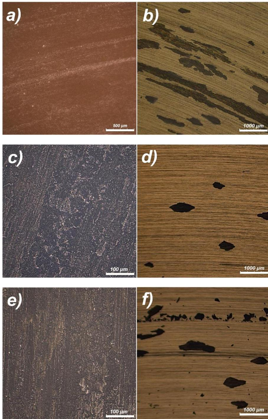
**Figure 5.** Optical microscope images of pin and disc wear surfaces under 10 N and 0.5 m/s a) Pure polyester pin, b) Pure polyester disc, c) 2% nano SiO<sub>2</sub> reinforced pin, d) 2% nano SiO<sub>2</sub> reinforced disc, e) 0.5 % nano ZrO<sub>2</sub> reinforced pin, f) 0.5 % nano ZrO<sub>2</sub> reinforced disc
