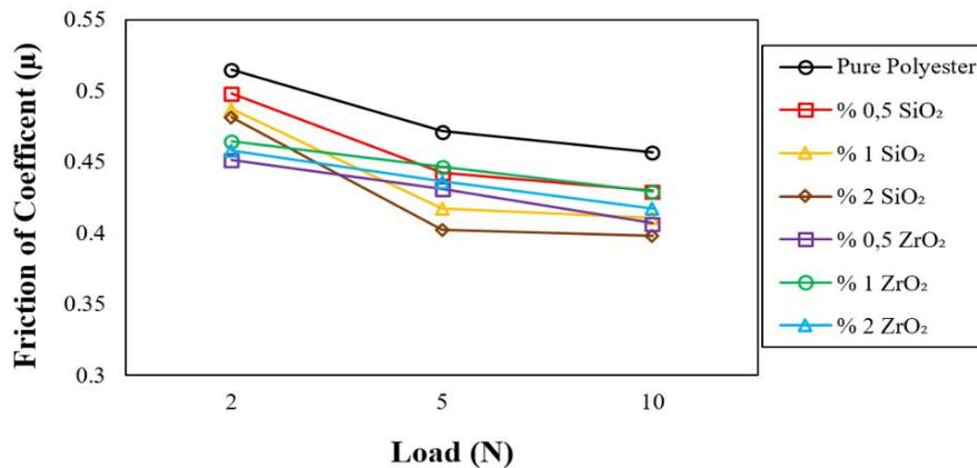
**Figure 1.** Variations of the friction coefficients of nanoparticle reinforced polyester composites at 0.5 m/s depending on the reinforcement ratio and the load
