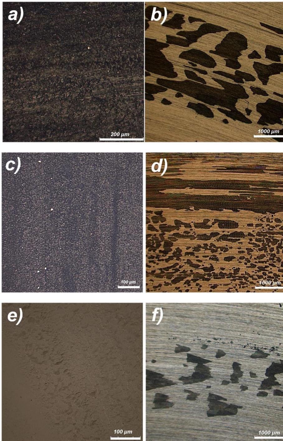
**Figure 6.** Optical microscope images of pin and disc wear surfaces under 10 N and 1 m/s a) Pure polyester pin, b) Pure polyester disc, c) 2% nano SiO<sub>2</sub> reinforced pin, d) 2% nano SiO<sub>2</sub> reinforced disc, e) 0.5 % nano ZrO<sub>2</sub> reinforced pin, f) 0.5 % nano ZrO<sub>2</sub> reinforced disc
