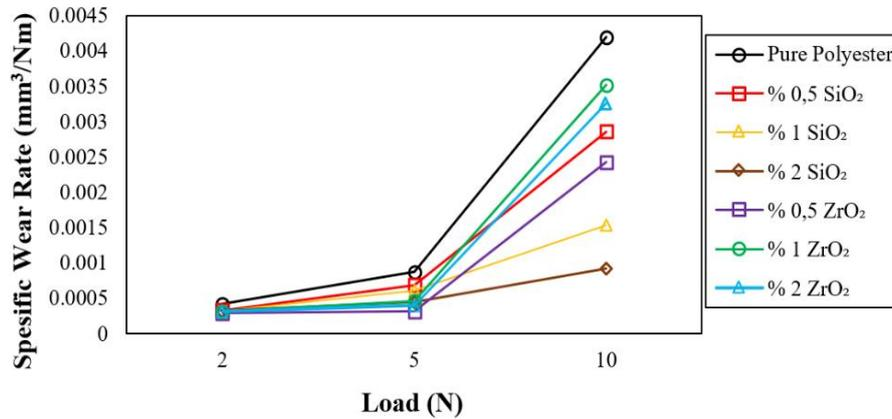
**Figure 3.** Variations of the wear rate of nanoparticle reinforced polyester composites at 0.5 m/s depending on the reinforcement ratio and the load
