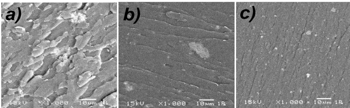
**Figure 8.** SEM images of nano SiO<sub>2</sub> reinforced polyester composites a) 0.5% SiO<sub>2</sub> b) 1% SiO<sub>2</sub> c) 2% SiO<sub>2</sub>
