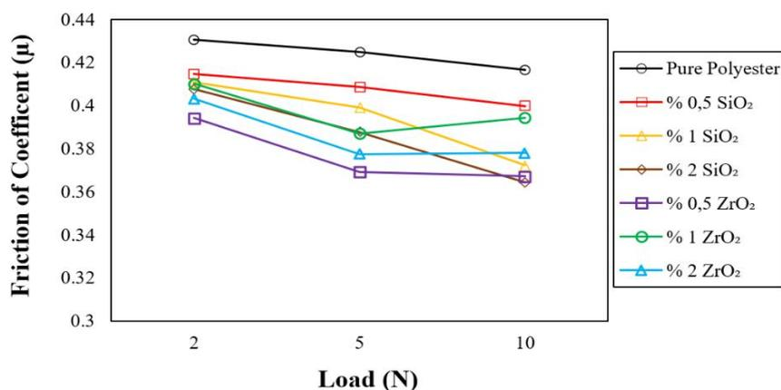
**Figure 2.** Variations of the friction coefficients of nanoparticle reinforced polyester composites at 1 m/s depending on the reinforcement ratio and the load
