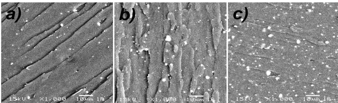
**Figure 9.** SEM images of nano ZrO<sub>2</sub> added polyester composites a) 0.5 % ZrO<sub>2</sub> b) 1 %ZrO<sub>2</sub> c) 2 % ZrO<sub>2</sub>
