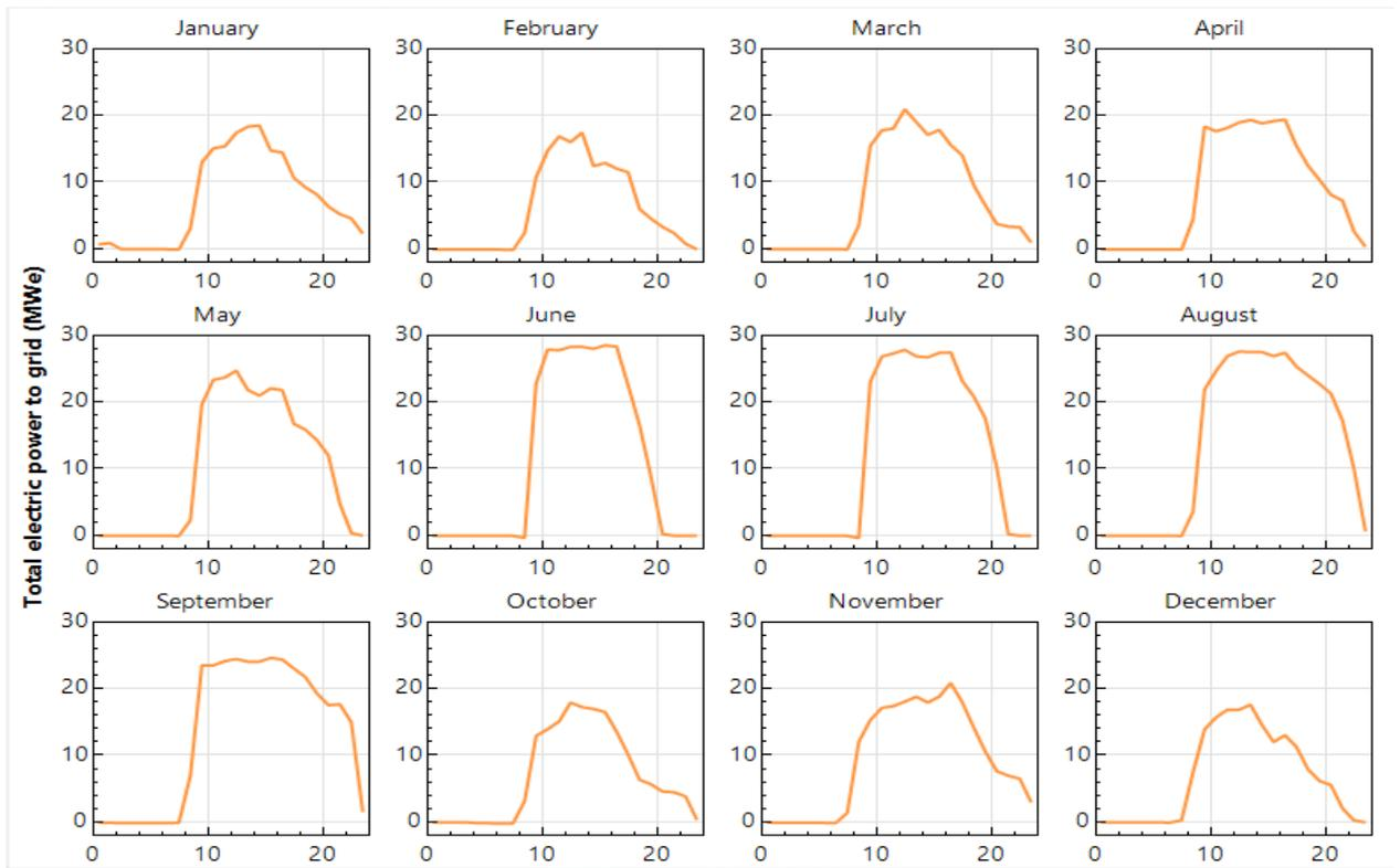
Fig. 3. Monthly electrical energy produced by the power plant
