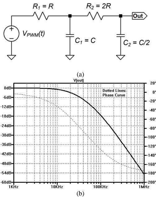
Figure 4. (a) Second order RC filter; (b) frequency response
