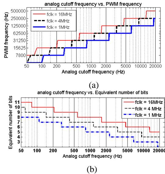
**Figure 5.** (a) Optimum PWM frequency vs. DAC output cutoff frequency (for the second order RC filter); (b) Equivalent number of bits when the optimum PWM frequency applied.
