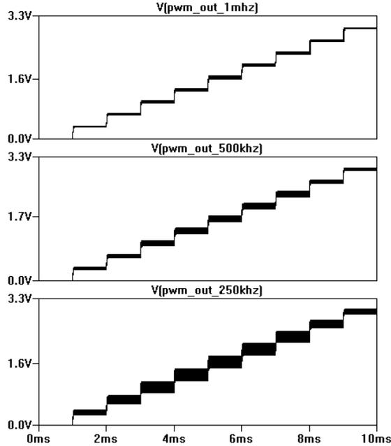
Figure 3. Analog output generated using various PWM frequencies
