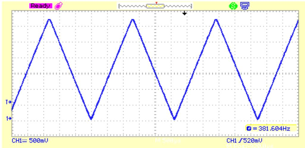
**Figure 7.** Digital oscilloscope snapshot of the PWM DAC with triangular wave generation
