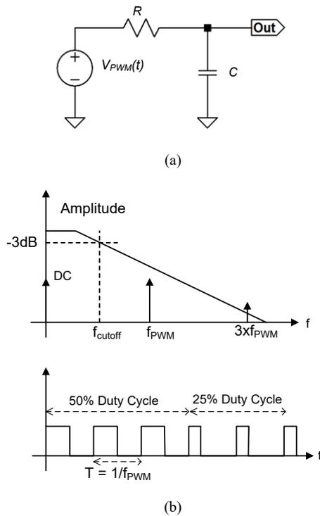
**Figure 2.** (a) PWM digital-to-analog converter; (b) frequency and time representation
