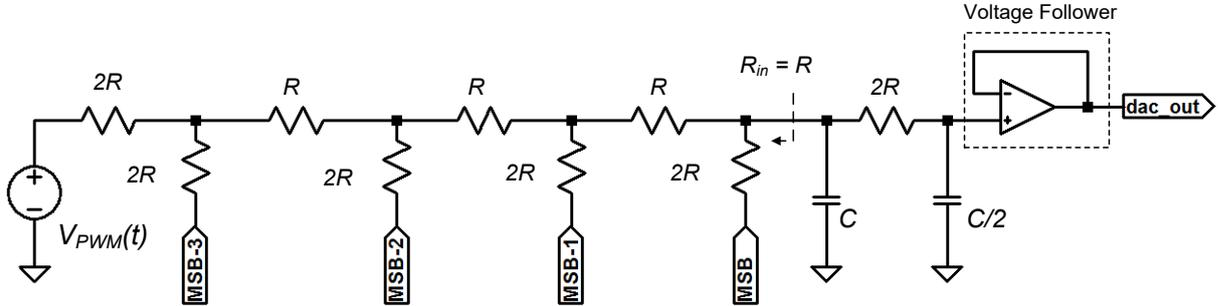
Figure 6. Hybrid DAC with second order RC filter
