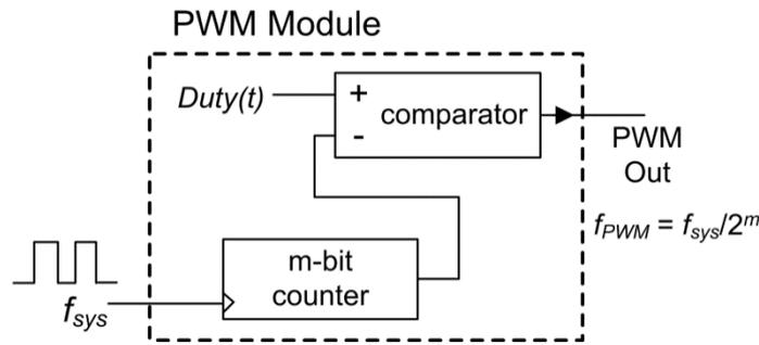
Figure 1. Pulse Width Modulator Structure
