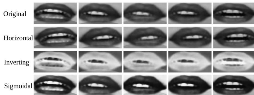
Figure 5. Data augmentation techniques applied on visual lip reading in Turkish dataset
