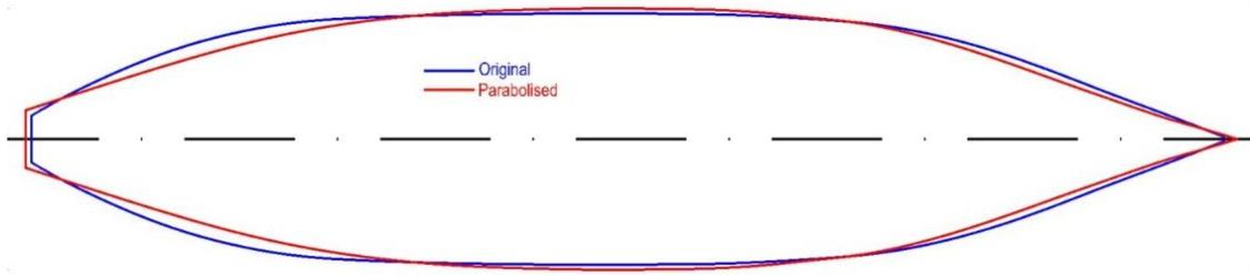
**Figure 2.** Beam increment at the loaded waterline.
