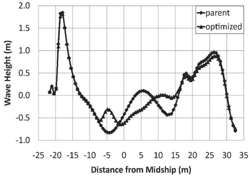
**Figure 9.** Comparative wave deformations around the hulls (V=13kn).
