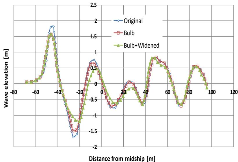
**Figure 7.** Wave elevations around the hull ( $V = 14.5$  kn).
