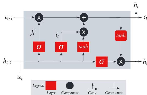
Figure 3. The structure of long-short term memory.
