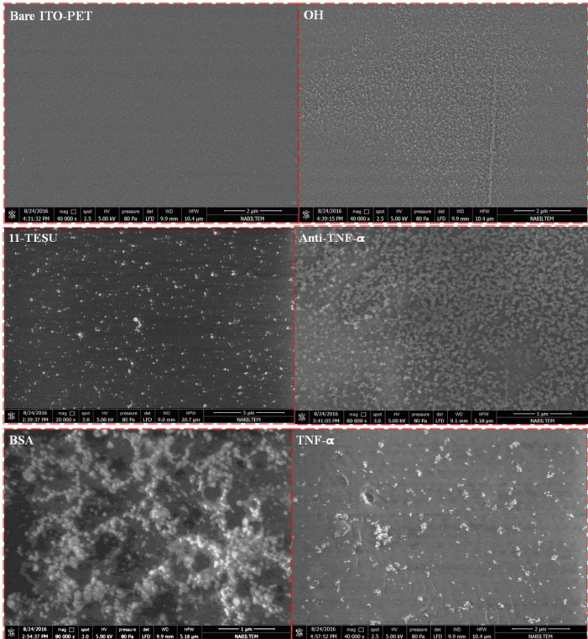
**Figure 4.** (1) SEM images of bare ITO-PET electrode, (2) OH, (3) 11-TESU, (4) Anti-TNF- $\alpha$ , (5) BSA, (6) TNF- $\alpha$ .
