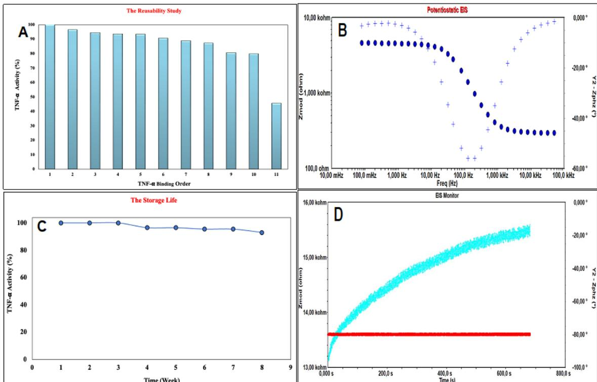
**Figure 3.** (A) Reusability, (B) Bode plot for SFI analysis, (C) Storage Life, (D) EIS measurement in the SFI.
