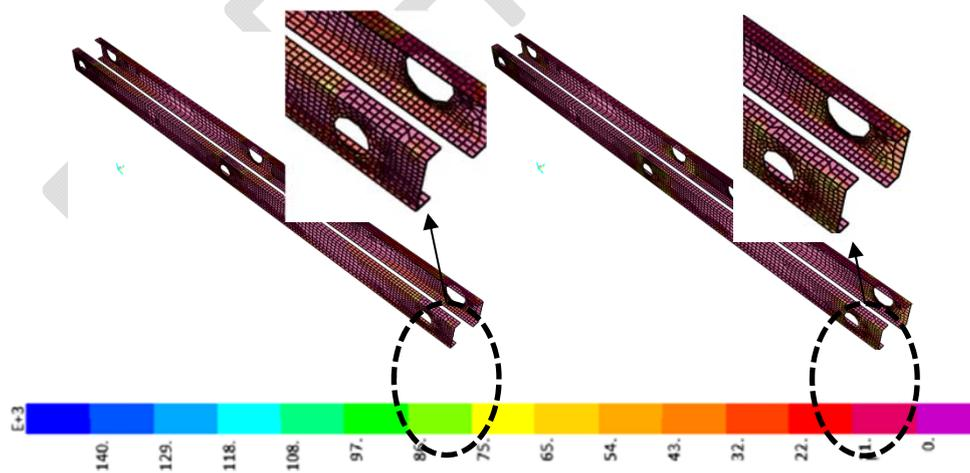
Figure 9 - Stress demands (kPa) obtained from finite element analysis of steel beams for 1-1 (left) and 2-2 (right) principal axes.
