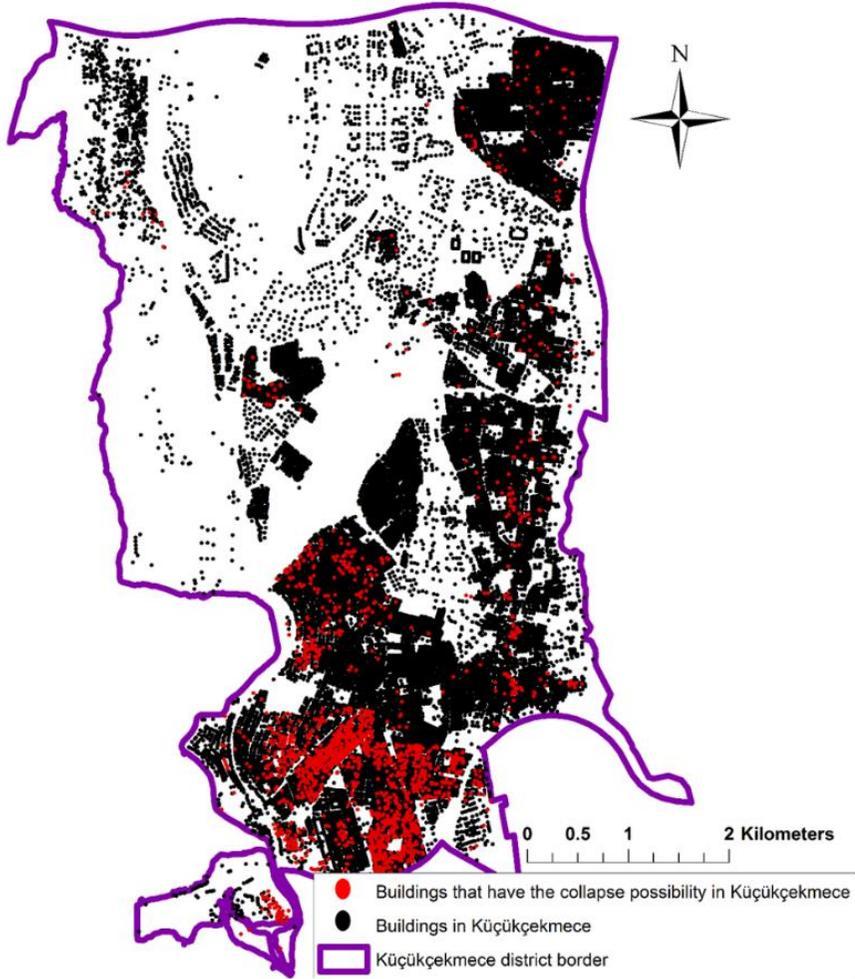
Fig 7. Buildings that have the possibility of collapse more than 30% according to Sa
