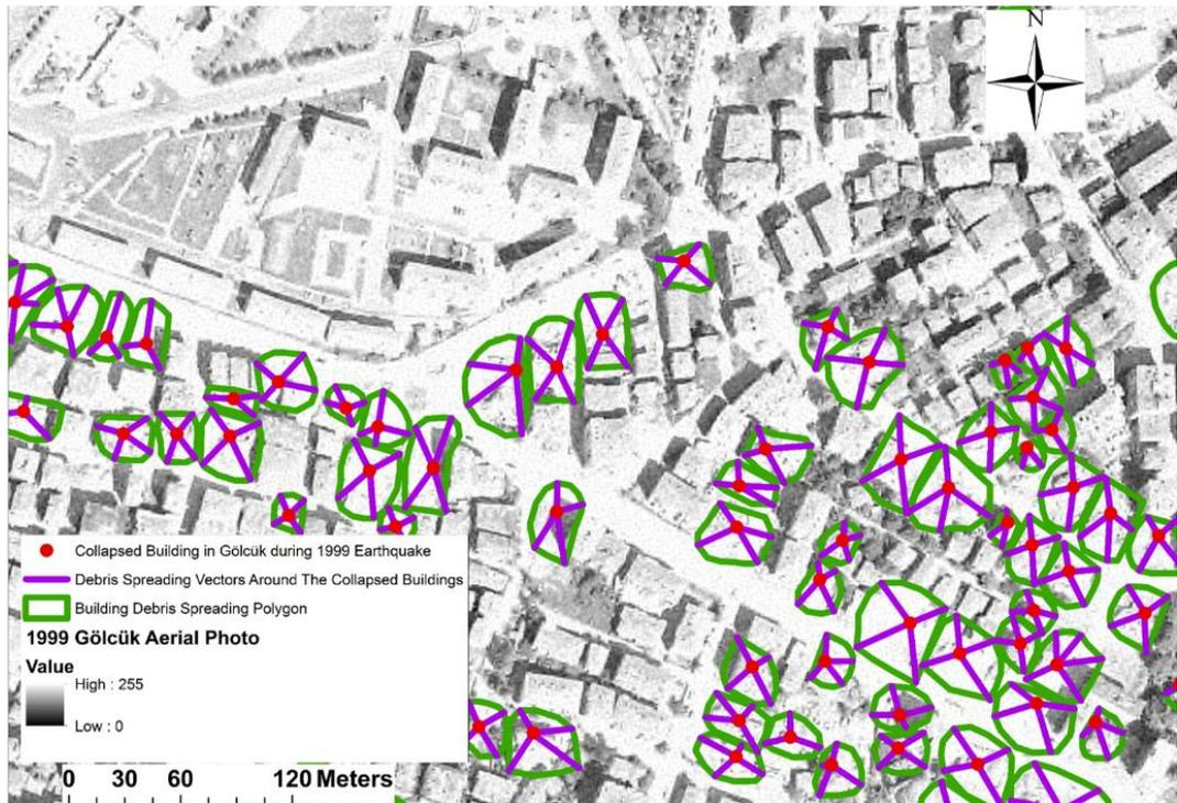
Fig 4. Building Collapse Directions in Gölçük
