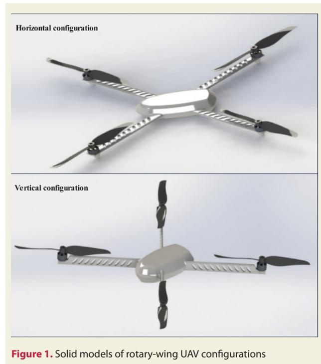
Figure 1. Solid models of rotary-wing UAV configurations
