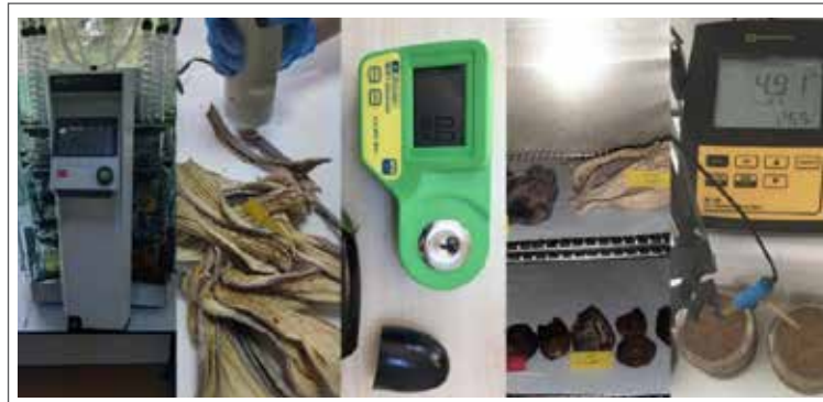
Figure 5. Equipment for analysis. A. used for oil determination; B. Spectropen colorimeter; C. Milwaukee MA871 refractometer device; D. Drying oven; E. pH meter. (Original)
