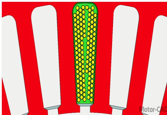
Figure-5: Winding definition for a Slot
