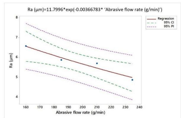
**Figure 8.** The effect of abrasive flow rate on the Ra when machining PLA material.
