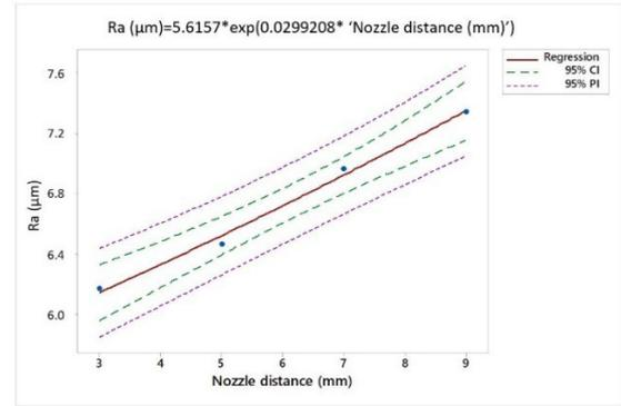
**Figure 11.** Surface roughness obtained in ABS material due to ND change.
