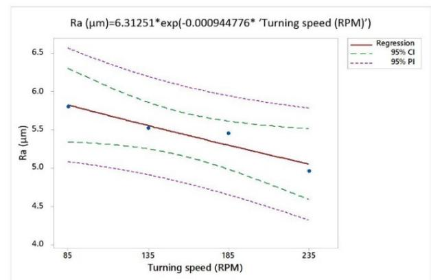
Figure 4. Influence of rotation speed on roughness when machining PLA material.
