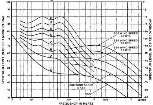
Fig. 3. Ambient noise due to shipping and wind (Ross, 2005: modified from Wenz, 1962)
