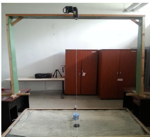
Fig.1. Experimental setup for an assessment of angular variation of emissivity. The FLIR T 650 SC was rotated about the sample and fixed at 30-degree intervals. Plastic APM DM 11 (up) and Metal APM M 16 (down) Positions.
