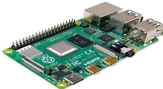
Figure 2. Raspberry pi 4 with 8 GB RAM
