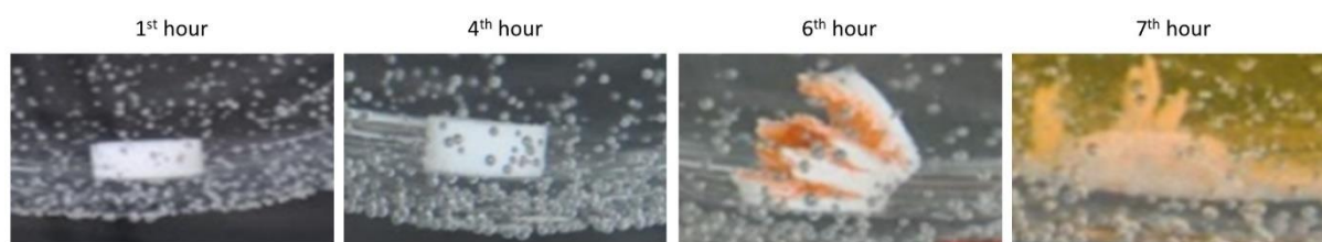
Figure 6. The images of CCT X-coded compression-coated tablets during in vitro dissolution tests
