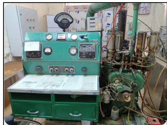
Figure 5: Single cylinder -test engine assembly for RON measurements.
