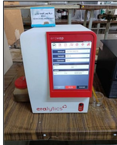
Figure 4: Reid vapor pressure apparatus.
