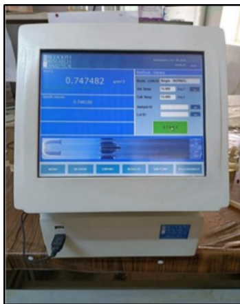
Figure 3: Digital density meter apparatus.
