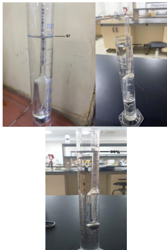
Figure 1: Determination of bioethanol Concentration using a gradual cylinder and hydrometer.
