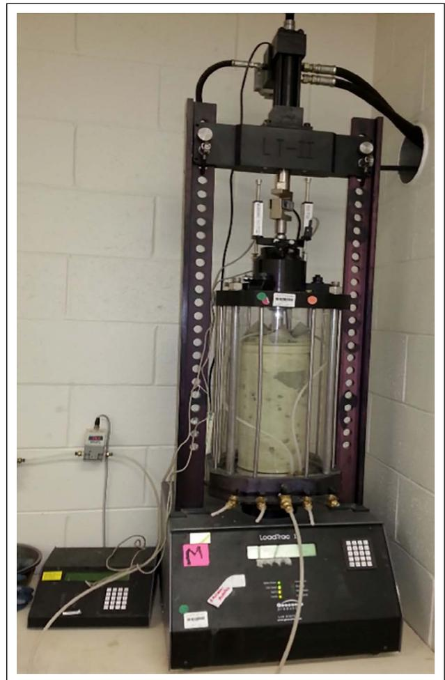
**Figure 2.** Resilient modulus test setup.
