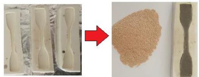
Figure 2. Polyester composite production scheme
