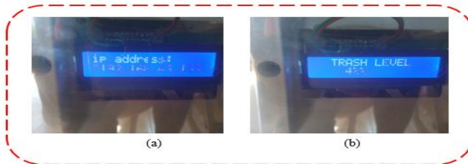
Figure 8. (a) Waste bin IP address (b) The waste bin’s percentage filled level
