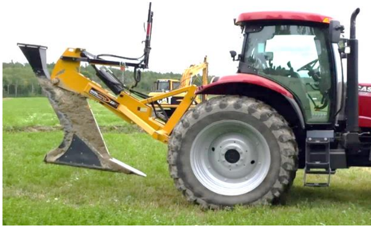
Figure 6. Plow-type trenchless machine.
